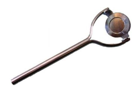
When placing on a magnetised test piece, magnetic lines pass trough the sectioned iron cylinder. The cuts on the iron cydinder will be visible when magnetic powder or magnetic ink is applied. Maximum indication direction is achieved by rotating the penetrameter about its axis. The field direction is perpendicular to the flaw at maximum indication.
